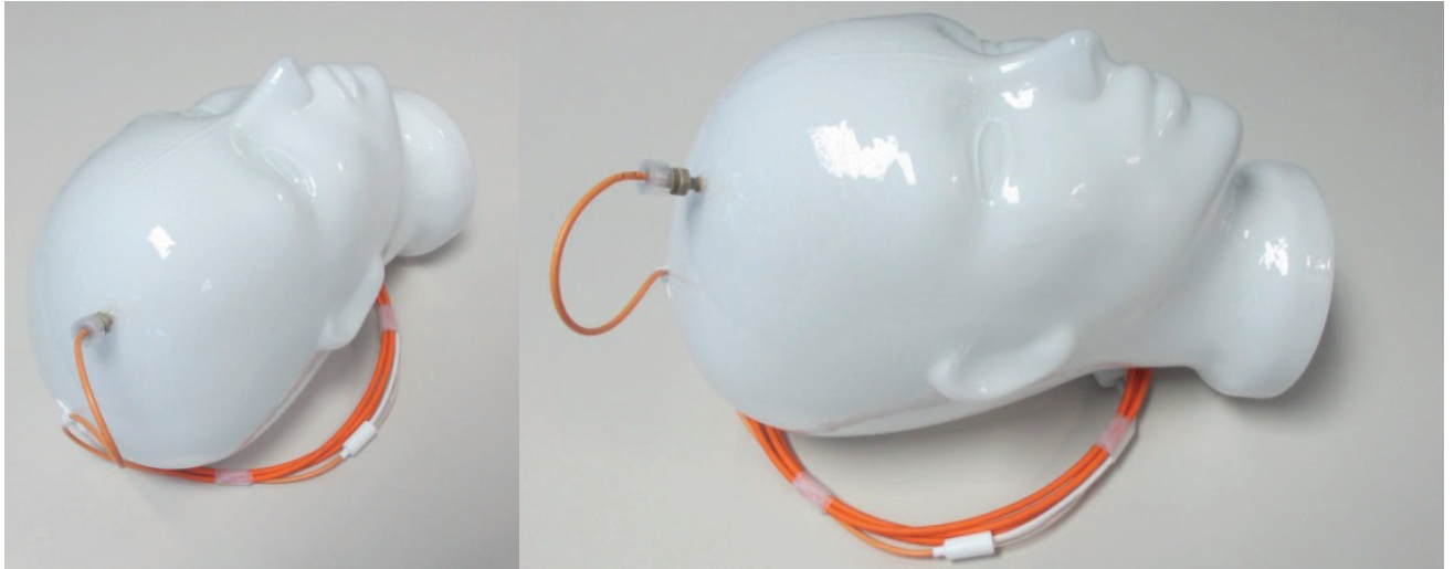
Picture 3: Configuration MRI – with coiled cable in tight head coils (e.g. Birdcage Coil)
